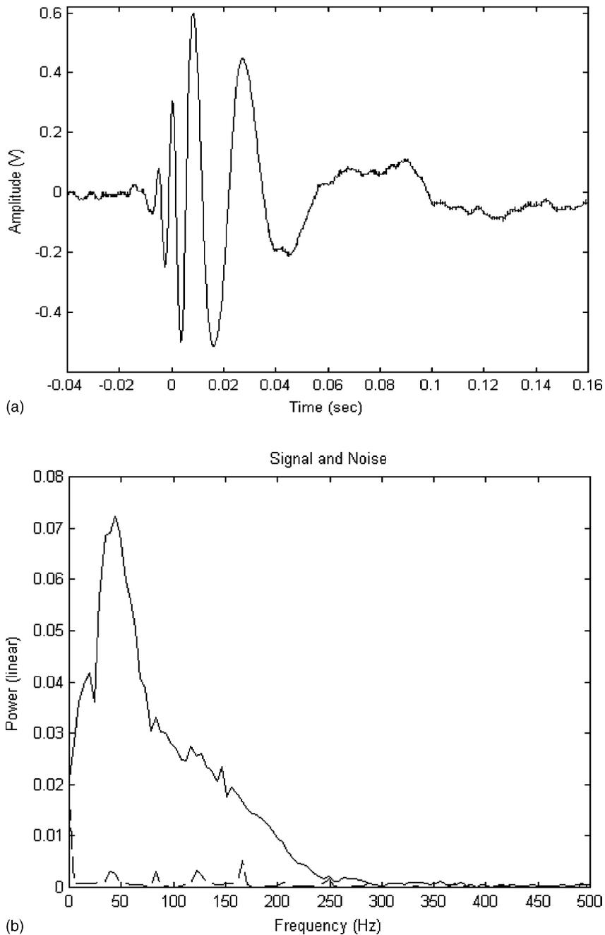
Fig. 4. Acoustical signal thought to originate from yellowfin tuna in the Monterey Bay Aquarium on 27 August 2000 (a), and its PSD (solid line) compared to that of the background noise (broken line) (b). In this example, the central frequency was 44 Hz, with an estimated SL of 114.5 dB re  $1 \mu\text{Pa}$  at 1 m.
