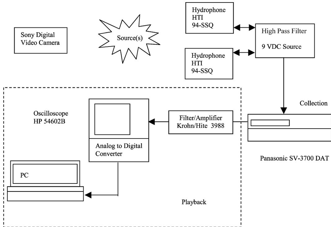
Fig. 2. Apparatus for audio and visual recordings of bluefin tuna at the Maricultura del Norte, Baja California.
