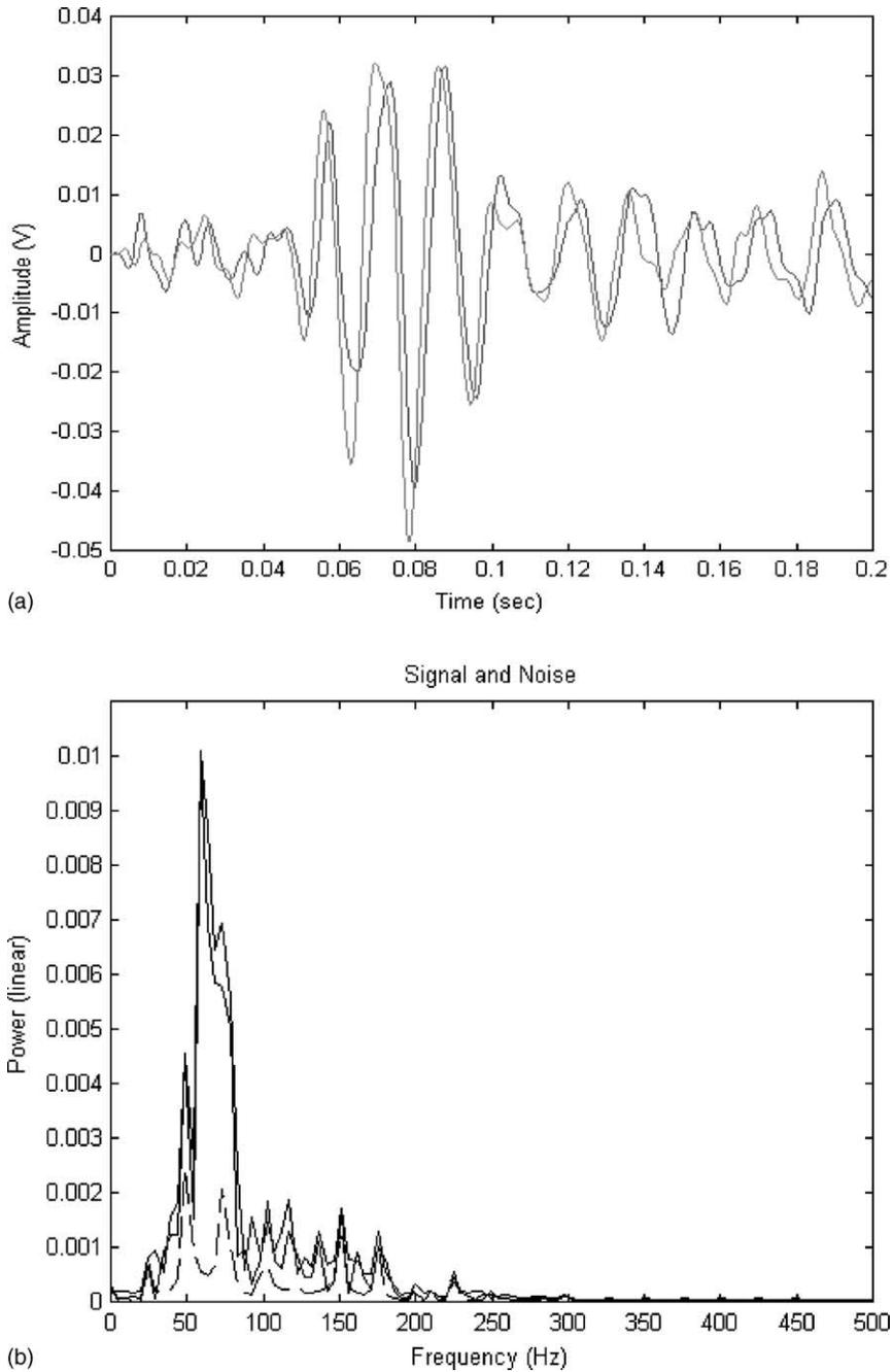
Fig. 5. Bluefin sounds recorded at Maricultura del Norte, 18 November 2000 using two hydrophones (a) and their PSD (solid line) compared to that of the background noise (broken line) (b). Signals were low-pass filtered (Butterworth, order 4,  $f_c = 600$  Hz). The estimated SL is 110.8 dB re  $1 \mu\text{Pa}$  at 1 m.
