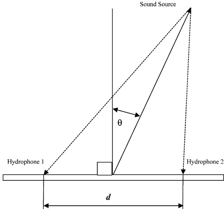
Fig. 3. Derivation of azimuth from phase difference. Azimuth is the angle of the source with respect to a normal bisector of two hydrophones and is described by Eqs. (2) and (3).
