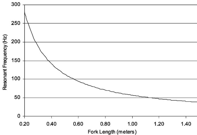
Fig. 8. Resonance frequencies for tuna having fork lengths ranging from 0.2 to 1.5 m. Magnuson (1973) derived a model for estimating spherical swim bladder radii from the fork lengths of yellowfin tuna (Eq. (5)). The resonance frequencies of gas bubbles of the same radii are described by Eq. (6) from Kinsler et al. (2000). If tuna sounds are the result of muscular action about the swim bladder, the resonant frequency of the swim bladder should determine the frequency of the sound pulses.
