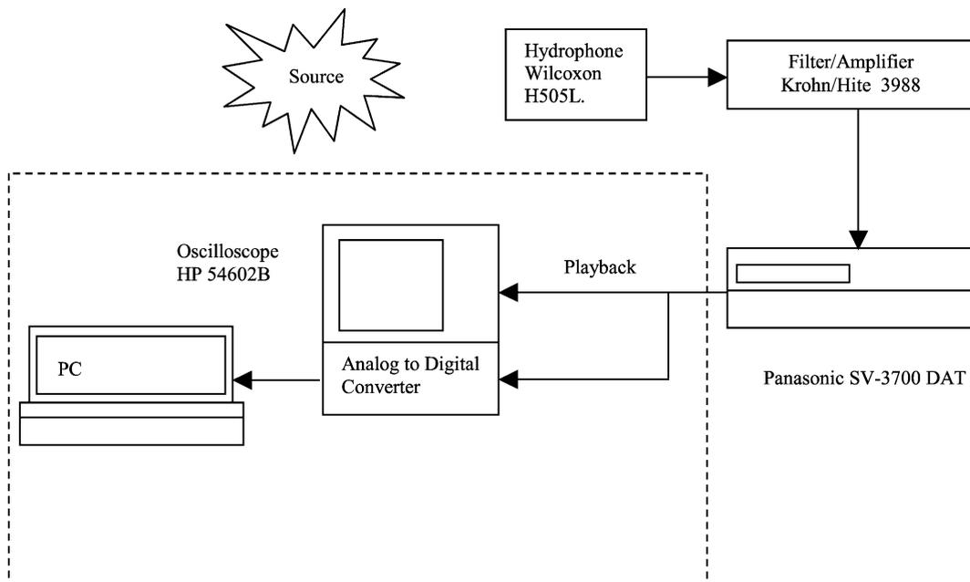
Fig. 1. Apparatus for recording tuna in the Outer Bay exhibit of the Monterey Bay Aquarium.
